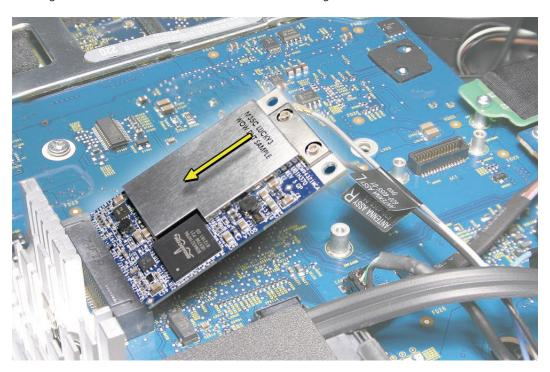
2. Connect the antenna cables to the connectors on the AirPort Extreme card. Note: The antenna cables might include an "L" or "R" tab near the connector end; however, you can disregard that because the cable position can be swapped without any change in performance. Replace the T6 screw.
